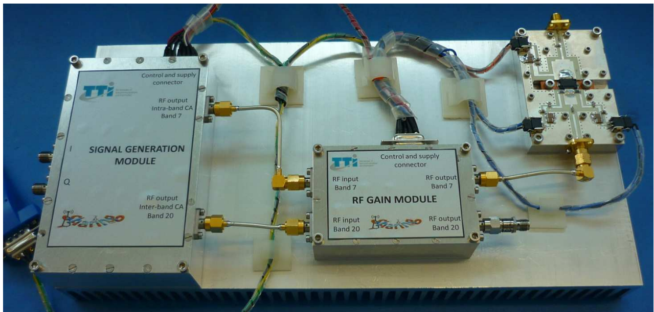
Figure 18 Reconfigurable and flexible bandwidth RF front-end prototype.
